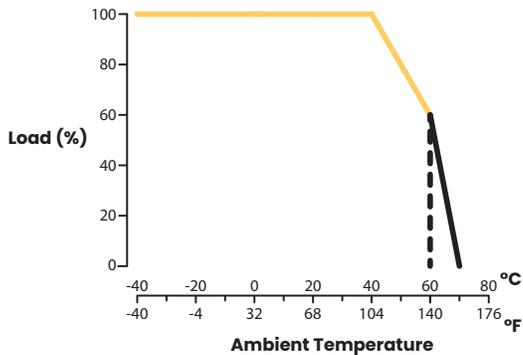
To extend Driver's life, derate according to the ambient temperature.
